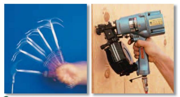
**The Best Tool?** A traditional hammer does not require electricity. Most carpenters prefer to use a pneumatic nailer for many nails. *If a carpenter used a hammer instead of a nailer to build a house, how might the cost of the project be affected?*
